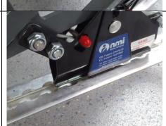
This shows a close up of the locked mechanism sitting on top of the groove.
