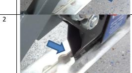
With one leg fixed into into the tracking, check the other leg. If it does not line up with the tracking, you may need to "guide" the mechanism into the groove. If this occurs, please inform the office that this has occurred and provide the seat number (ie seat JBY-05).
