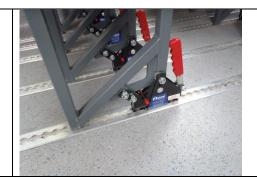
Inspect both front legs and both rear legs are in the tracking.
