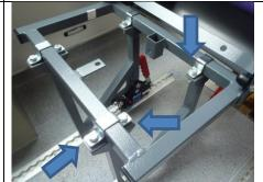
Using a 13mm socket or spanner, loosen the three bolts on  ${\bf one}$  side of the seat.
