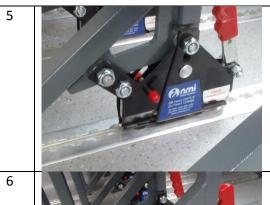
Note that this handle has been lifted, and the seat mechanism locked, but the mechanism is locked outside the groove – THIS SEAT IS DANGEROUS AND IS LIABLE TO FAILURE, POSSIBLE **INJURY** OF PASSENGERS IS LIKELY
