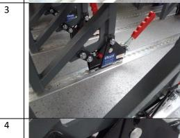
Care should be taken when locking the seat fixing mechanism. As pictured, the farthest mechanism has not dropped into the groove prior to lifting the handle
